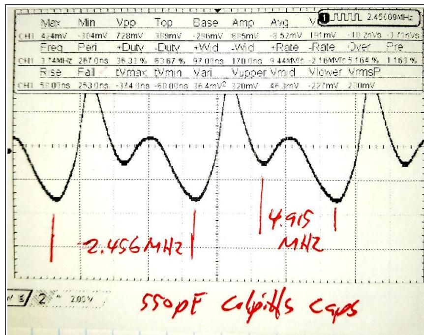
I changed the Colpitts capacitors to 440pF and there was no change in the results for 4.915MHz crystals except the tolerated Vcc was below 3.9V. The 9MHz and 11.052MHz crystals worked fine. The 11.052MHz crystals could take up to 10.2Vcc before becoming unstable.
